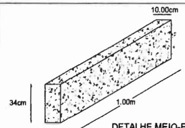
DETALHE MEIO-FIO SEM ESCALA
