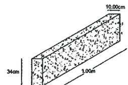
DETALHE MEIO-FIO SEM ESCALA
