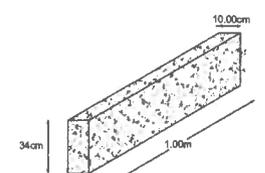
DETALHE MEIO-FIO SEM ESCALA
